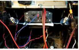
OF THE RAB150 BRACKET WHERE THE AMPLIFIER WILL STAY, PLACE A PIECE OF PAPER (LIKE THE GUIDE YOUR READING) ON TOP OF THE VELCRO THAT IS NOW ATTACHED TO THE RAB150 BRACKET. NOW SLIDE THE AMPLIFIER INTO PLACE. THE VELCRO WILL NOT ATTACH TO ITSELF UNTIL YOU REMOVE THE PAPER. WE SUGGEST YOU KEEP THE PAPER THERE UNTIL ALL CONNECTIONS AND ADJUSTMENTS ARE COMPLETE AND YOU ARE READY TO WRAP UP THE INSTALL AND PUT THE FAIRING ON.
