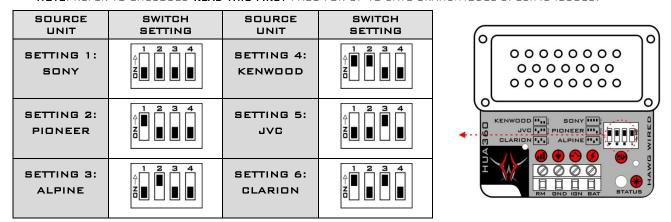
THE DIP SWITCH IS COVERED BY A PROTECTIVE MEMBRANE. THE SWITCHES CAN BE TOGGLED ON/OFF WITH THE MEMBRANE INTACT, OR IF DESIRED THE MEMBRANE CAN BE REMOVED WITH TWEEZERS OR NEEDLE NOSE PLIERS.
