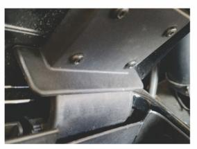
**STEP 1.** Clean hinge using alcohol pad. Let area dry or wipe with clean cloth.
