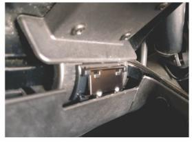
**STEP 5.** Apply pressure to the detent to ensure adhesion of the double stick tape to the hinge.
