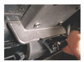
**STEP 3.** Line up detent device in the middle of the hinge with the top registered firmly against lip of hinge. Refer to the photo showing detent being held at an angle against the lip. **STEP 4.** Press detent onto hinge while keeping top of detent against the lip of the hinge. Pull door up a bit more if front lip of detent hits the back of the glove box. This is normal.
